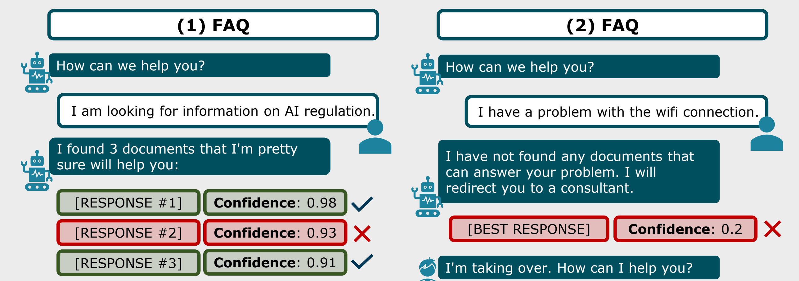
Fig. 6: Illustrative example of how MAPIE approaches NLP (Information Retrieval / Topic Detection / Task-oriented Chatbot): (1) It allows to find the most relevant answers to the user without mental overload by selecting only the most reliable answers. (2) It avoids the frustration of the user if it considers that no answer is pertinent by redirecting him to a human.
